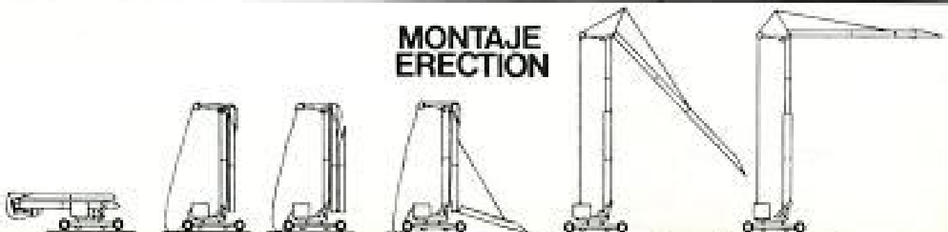
REMOLCADA POR CAMION O TRACTOR TOWING BY TRUCK OR TRACTOR ① semmontada con lastre (tren F 12/21) semi-erected with ballast (towing unit F 12/21)
